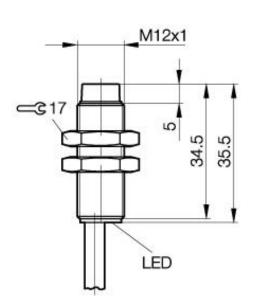
**Inductive Sensors** BES 516-357-E4-Y-03 M12x1 x 35.5 normally-open Sn=4mm unshielded
